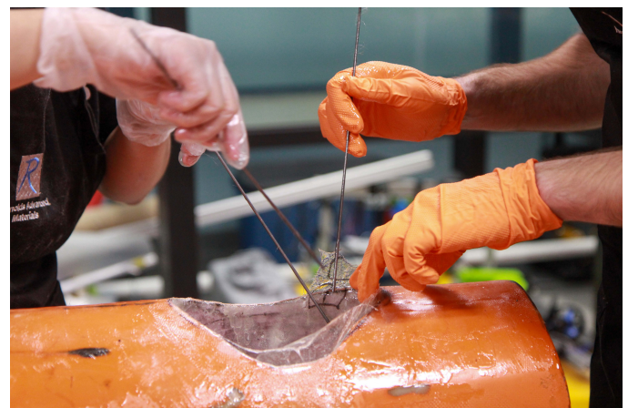
Figure 8: Difficult-to-access geometry required us to pre-soak the fiberglass strips and place them using welding rods.
