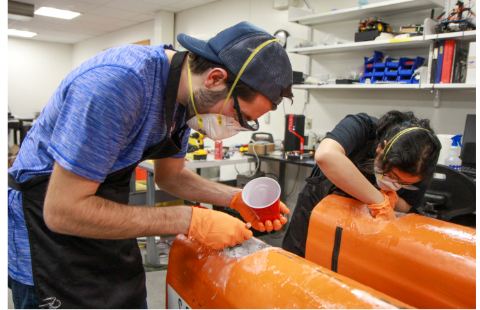
Figure 6: Epoxy is painted onto the fiberglass strips for sections with simple geometry.
