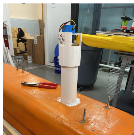
Figure 10: Final assembly of thruster pod embedded within the hulls.
